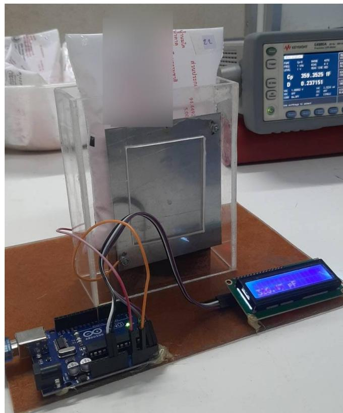
Figure 2. The proposed capacitance measuring device.
